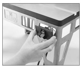
Figure 9. Installing the switch.
